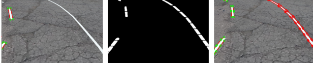
Fig. 7. Curve Detection Using DeepLSD.
